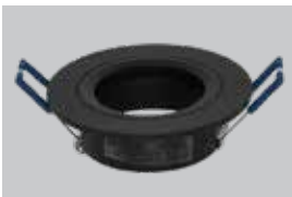
R211 BN717 - AL Downlight Fixture Black • Flat • Fixed CNC Aluminium Ø80 x H25 / Cut 65 - 70
